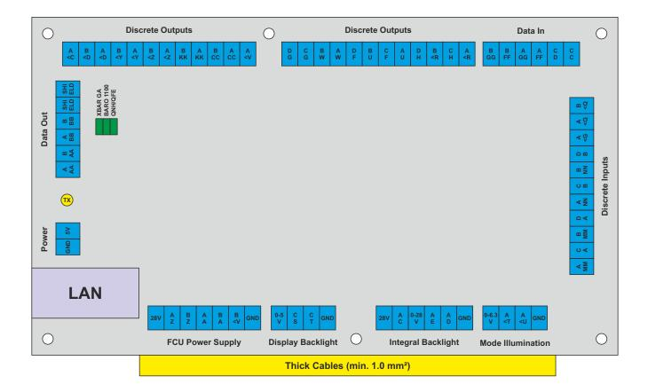
Connect the board with a LAN cable to your local network. Connect a 5 V power supply to the board and it will power up. By default the board will try to retrieve an IP address by DHCP. Check your router which IP it got. You may open that IP and change the network settings if you like (if you need an username or password just ignore it / press enter) or leave it as it is.
